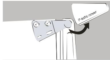
5) To install the bracket on the left side of the appliance, screw the two screws through the bracket and into the top of the appliance. Slide the door back on to the top hinge. Ensure the door is face up. Replace the plastic cover on the top bracket by pressing down until it clicks into position.
